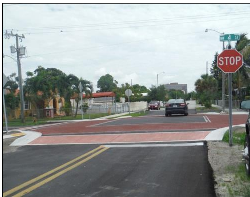
Figure 11. Example Tabled Intersection
